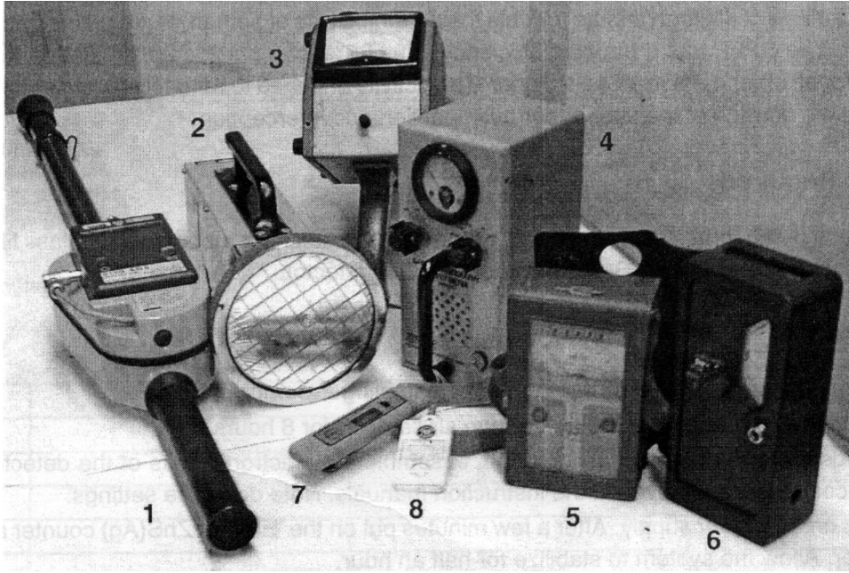
Fig. 4.6 Photographs of different radiation monitors. (1. Teletector, 2. Alpha monitor, 3. Gun monitor, 4. Radiation survey meter, 5. Minirad survey meter, 6. Bicon survey meter, 7. Digi dose personal monitor and 8. TLD badge).
