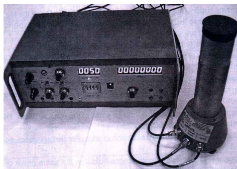
Fig. 3.6 NaI(Tl) detector and single channel analyzer system.
