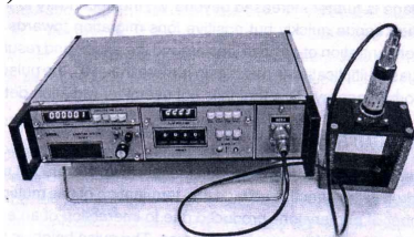
Fig. 1.6 Photograph of GM Counting system.
